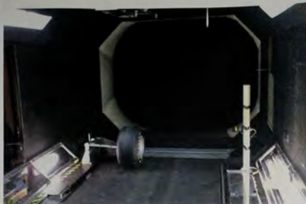
While the design development for the F1 project was all CFD the validation work on isolated wheels and tyres was carried out in the wind tunnel at Southampton University
