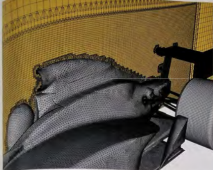
The surface mesh and a slice through the volume mesh on the 2004 Dallara IndyCar
