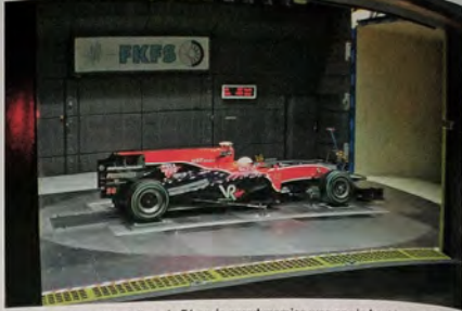
Some validation of the full-scale F1 car's aerodynamics was carried out in the FKFS Stuttgart facility in Germany. Flow visualisation validation at the track was also used
