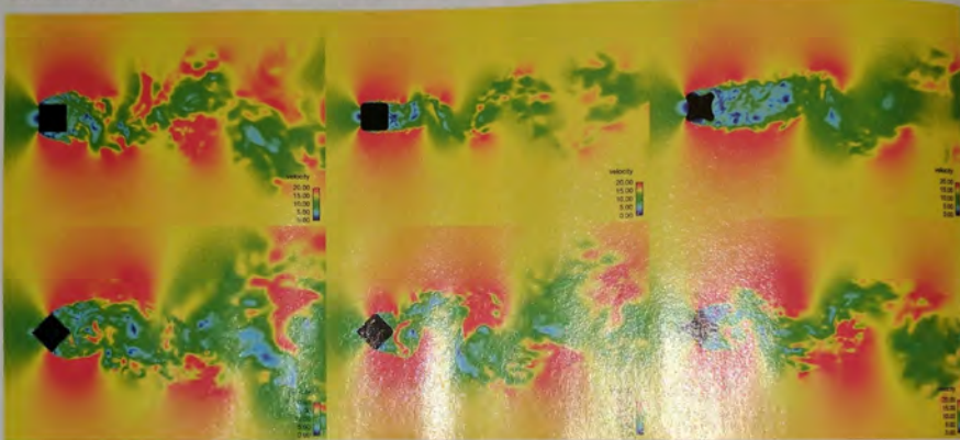
Studying various tall cylinder shapes helped refine the CFD methodology for architectural flow simulations. It was only much later that WR did work such as this in a wind tunnel
