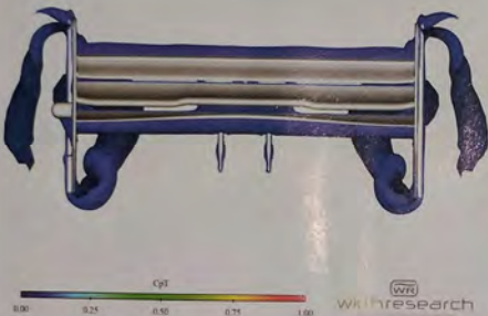
Productivity was increased with the use of sub-models; such as this rear wing with end plate assembly and mounting plates. The results correlated closely with full car models
